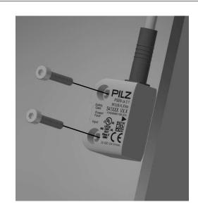
3. Attach the screws for the actuator, leaving a distance of 3 ... 6 mm between the screw head and plate.
